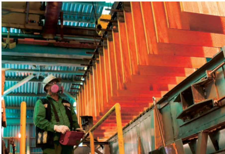
Above: Washing down copper cathodes in the solvent-extraction/electro-winning plant at Mantos Blancos in Chile
